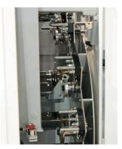
The wheel loading system with a HSK50 clamping system can handle and manage up to 14 prepared wheel packs.
