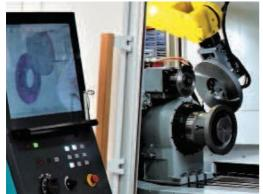
With a robot, (max load 20 Kg) the automatically off loading / loading of tools can be realized.
