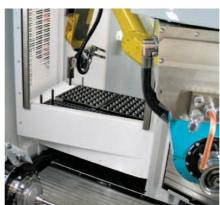
The Fanuc robot, double gripper system can manage a 2 or 4 pallet system with tools..
